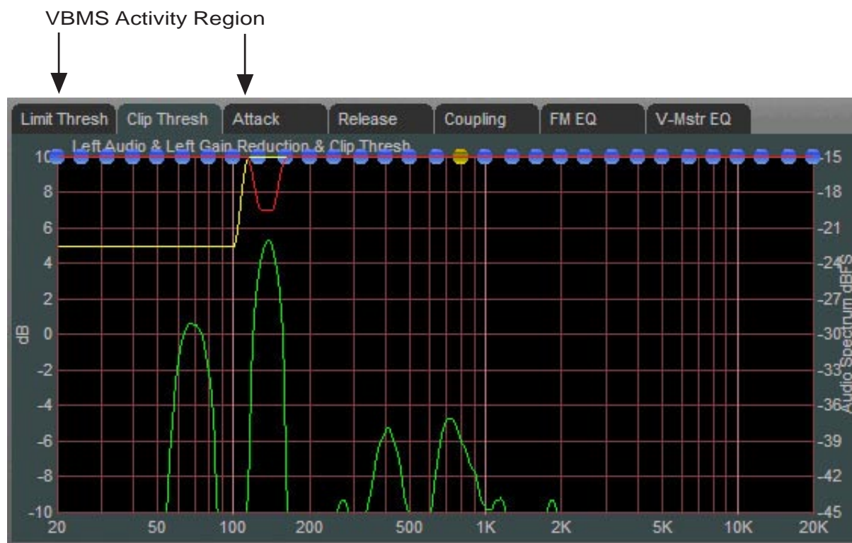
VBMS Activity Display - 20Hz up to the VBMS Frequency Setting
